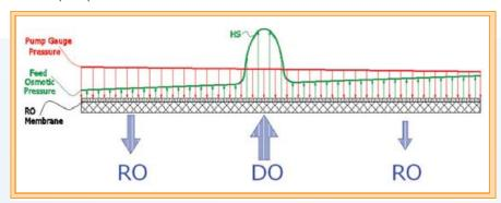
In the clean-in-place tank, a 25% saline solution is added with an osmotic pressure of 2800 psi. For 10 - 15 seconds, this saline solution is injected into the feed water stream. The osmotic pressure is much higher than the hydrostatic pressure of the feed water pump, reversing the osmotic flow and back washing each membrane in succession like a vacuum cleaner.
